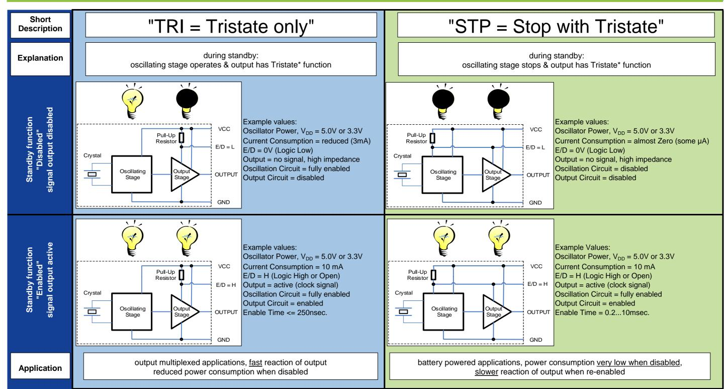
\*Tristate Tristate means that the output can have 3 states: High or Low when enabled / High Impedance if disabled
