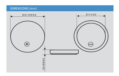
Note: Capacity 550mAh is obtained at standard cc load to 2.0V at 23  $^{\circ}\text{C}.$
