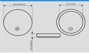
Note: Capacity 550mAh is obtained at standard cc load to 2.0V at 23  $^{\circ}\mathrm{C}.$
