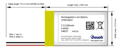
Thickness (max): 2.8 mm (delivery status) 3.0 mm (after cycling)
