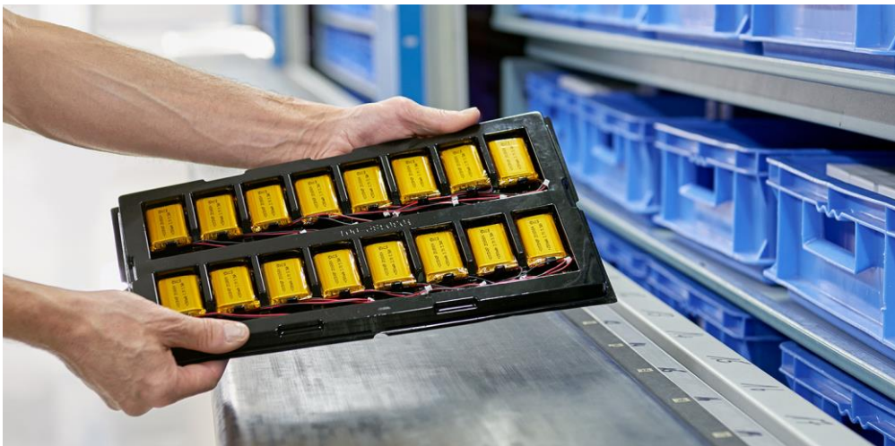
fig. 3. Suitable trays are used to transport lithium-polymer cells safely. Image: Jauch
