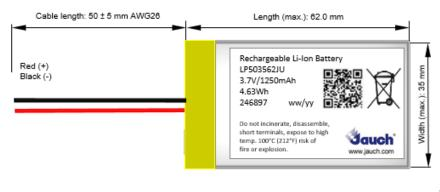
Thickness (max.): 5.0 mm (deliver status) 5.4 mm (after cycling)
