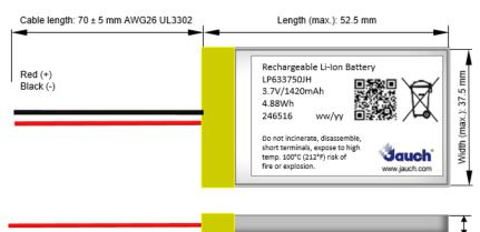
Thickness (max.): 6.3 mm (deliver status) 6.8 mm (after cycling)
