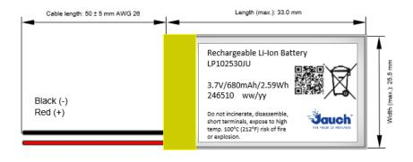
Thickness: (max.): 10.2 mm (delivery status) 10.8 mm (after cycling)
