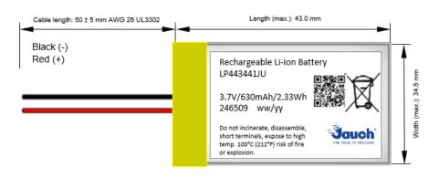
Thickness: (max.): 4.6 mm (delivery status) 4.9 mm (after cycling)
