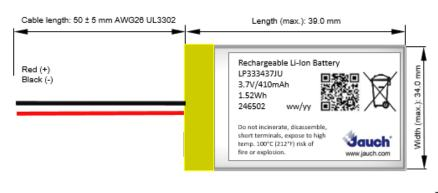
Thickness (max.): 3.5 mm (deliver status) 3.7 mm (after cycling)
