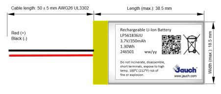
Thickness (max.): 5.6 mm (deliver status) 6.0 mm (after cycling)
