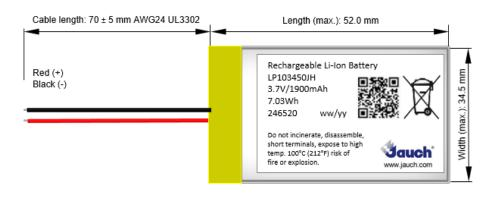
Thickness (max.): 10.0 mm (deliver status) 10.8 mm (after cycling)
