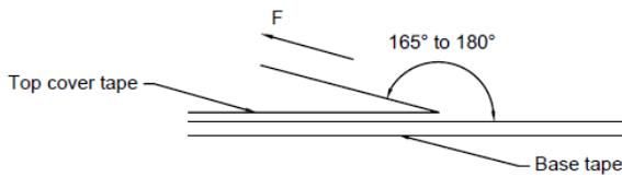
The force for tearing off cover tape is 10 to 130 grams in the arrow direction under the following conditions
